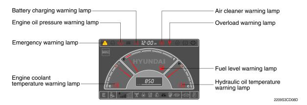
\* Each warning lamp on the top of the LCD pops up on the center of LCD and the buzzer sounds when the each warning is happened. The pop-up warning lamp moves to the original position and blinks when the select switch is pushed. And the buzzer stops. Refer to page 3-10 for the select switch.
